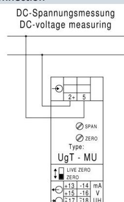
For devices with frequency output further outputs not available. Terminals +13 and -14 are the frequency output.
