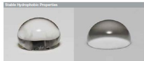
Water droplet on a dirty silicone coating.
