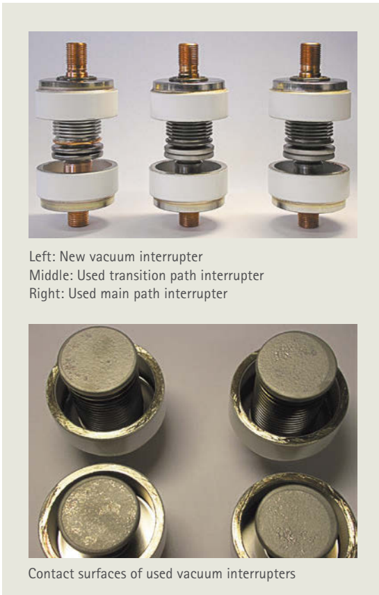
Fig. 18: Opened vacuum interrupters after 300,000 EAF-operations
