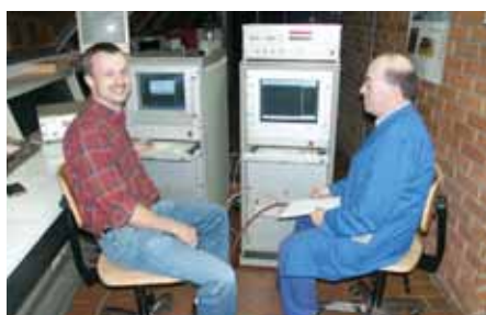
Calibration of the voltage measuring system of a mobile AC test system in Saudi Arabia
